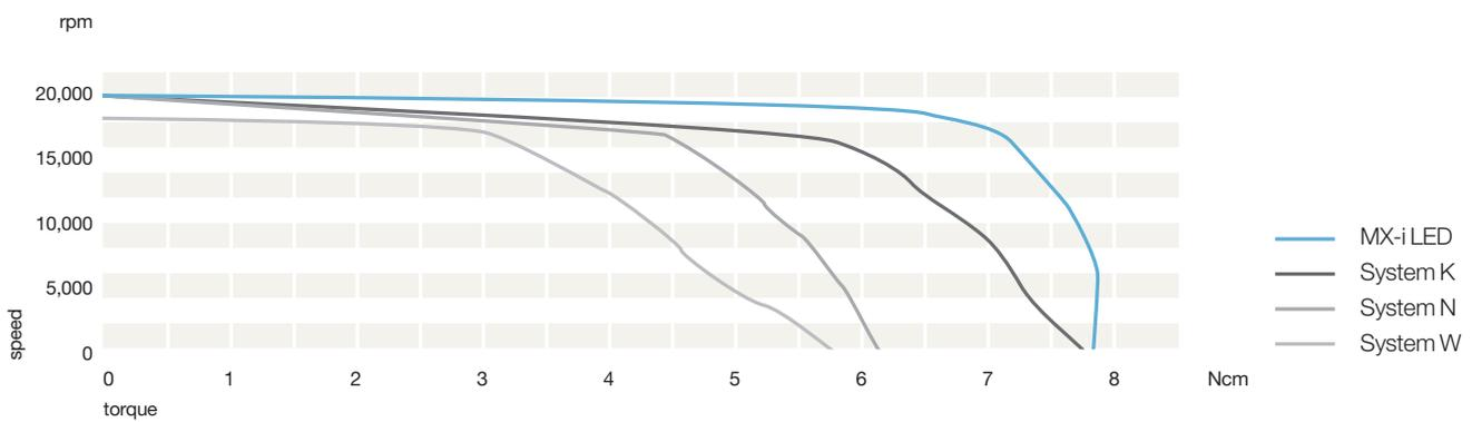
The MX-i LED micromotor is a model of stability. At both high and low speeds, the new MX-i LED offers you ideal working comfort. With its high level of output torque, the MX-i LED is just simply the most powerful micromotor on the market. Depending on the torque needed, the power is automatically regulated and stabilised electronically. Accordingly, the speed is kept constant throughout the operation.
